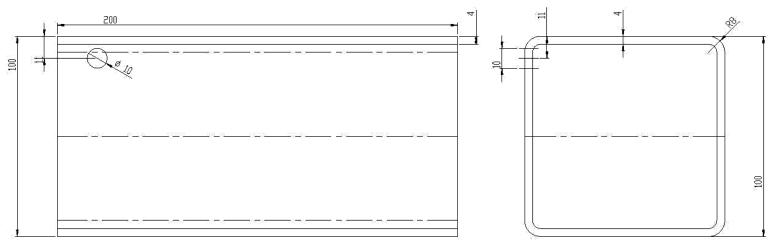
When a hole is cut into the radius of a box section the cutting head cuts perpendicular (XA) when the material is rotated the laser causes an eyedrop effect where the radius of the box section is (below left). The cutting head can be manipulated in the B axis to cut (XY) avoiding the eyedrop (below right), this process takes a longer time and cannot always be achieved. **Programmers default to hole cutting as XA**, XY needs to be specified at the point of quotation.
